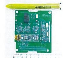
Figure 8. Electronics for the SIGMA fluxgate magnetometer.
